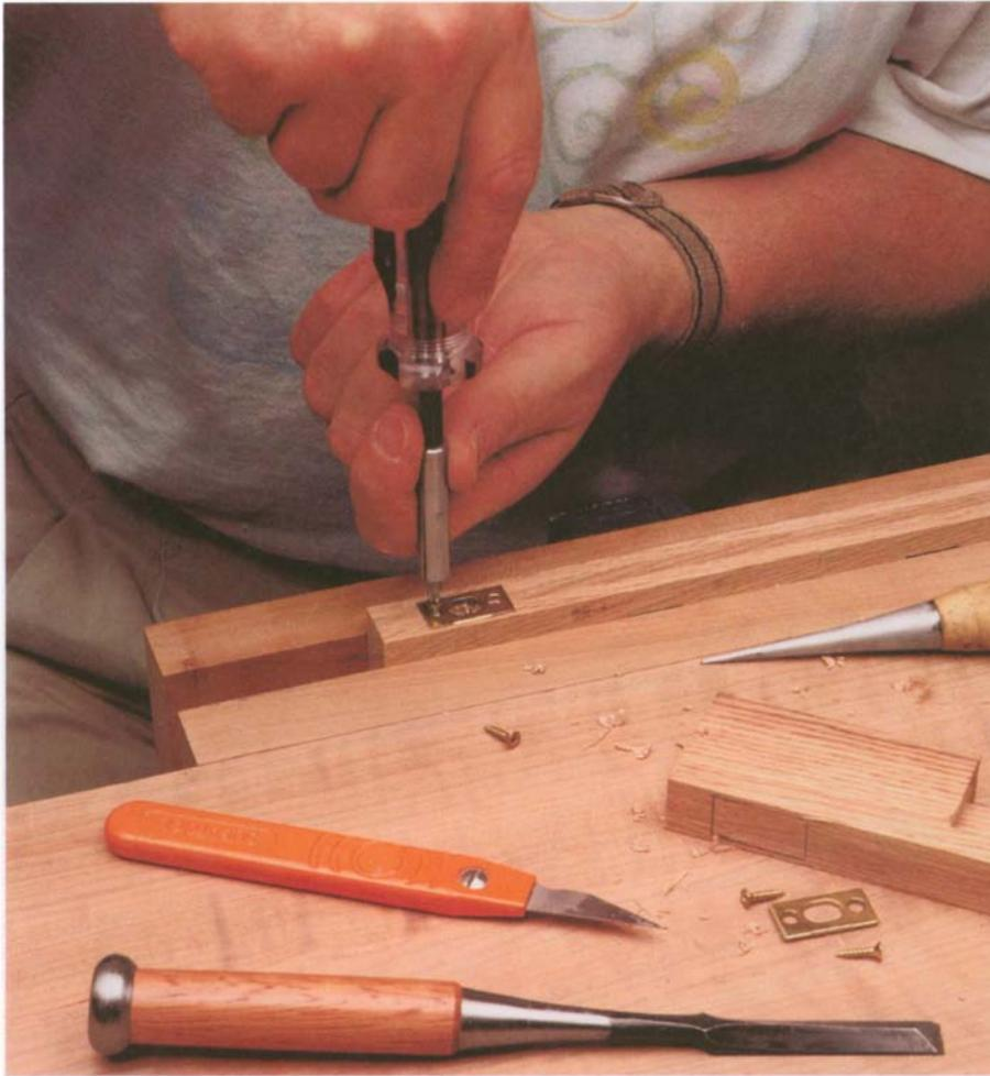
**PHOTO D:** Install hanger hardware flush with the back side of the uprights.
