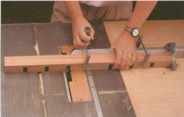
**PHOTO A:** Cut the shelf notches in the uprights with a dado blade on the table saw.
