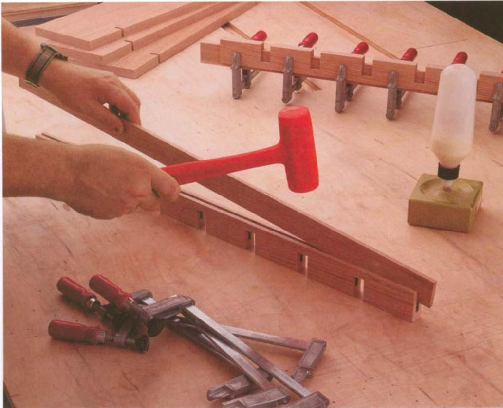
**PHOTO B:** Gently tap overlong splines into the uprights. Clamp the uprights across their faces so they don't bulge while the glue sets.
